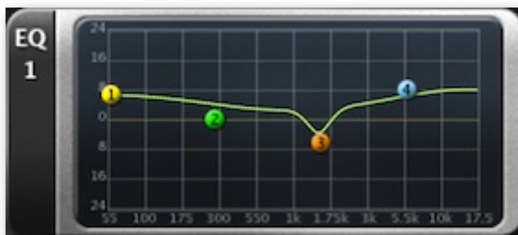
Equalizer module, bass+treble boost, dip around 1.5 kHz
